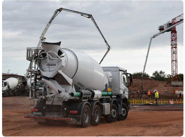
Reference: mixer and boom pump setup for a pour this size.
